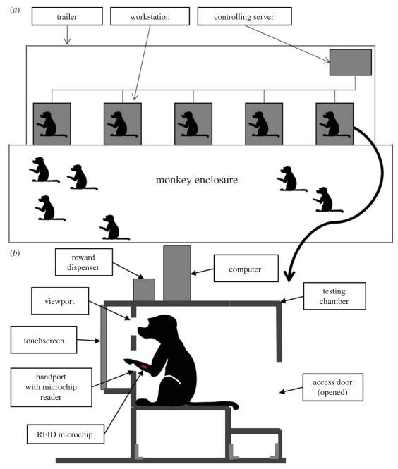
**Figure 1.** Principle of the self-testing apparatus. (*a*) Bird's-eye view of the enclosure and the trailer containing the workstations. (*b*) Schematic of a baboon working at a workstation. (Online version in colour.)
